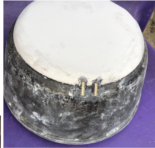
Plaster to cover electronics
