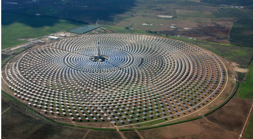
Solar farm with energy stored in molten salt tower
